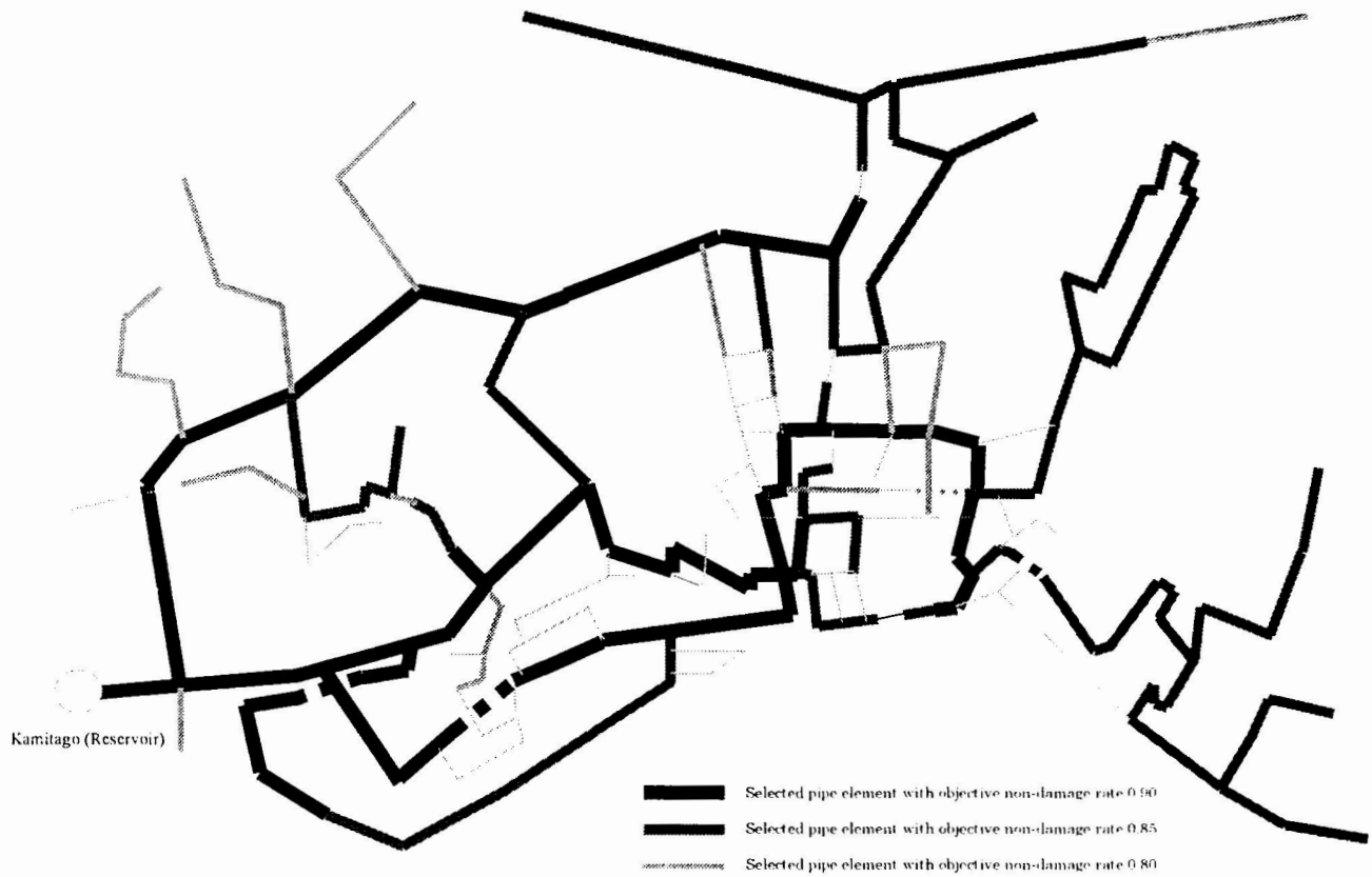
Figure 3 Selected pipe element
